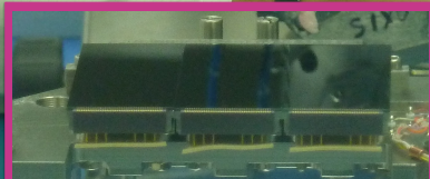
The new e2v detector array, installed in the GMOS-N focal plane and ready to go back in the dewar.
