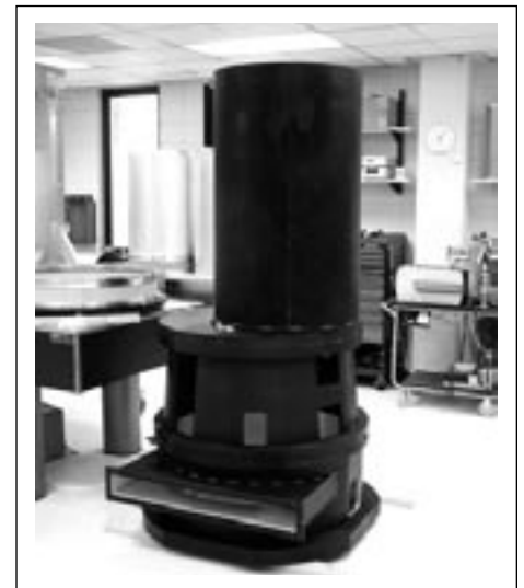
Figure 2: The FLAMINGOS-2 camera dewar vacuum jacket, dewar spacer ring, and MOS dewar vacuum jacket, stacked to simulate the completed instrument.
