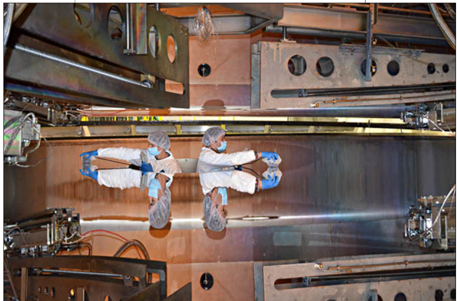
Figure 3. The Gemini North 8.1-meter primary mirror is inspected inside of the coating chamber.
