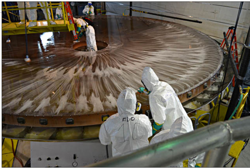
Figure 7. The 8.1-meter Gemini primary mirror being washed (after stripping of old coating) and prior to receiving a new protected silver coating.
