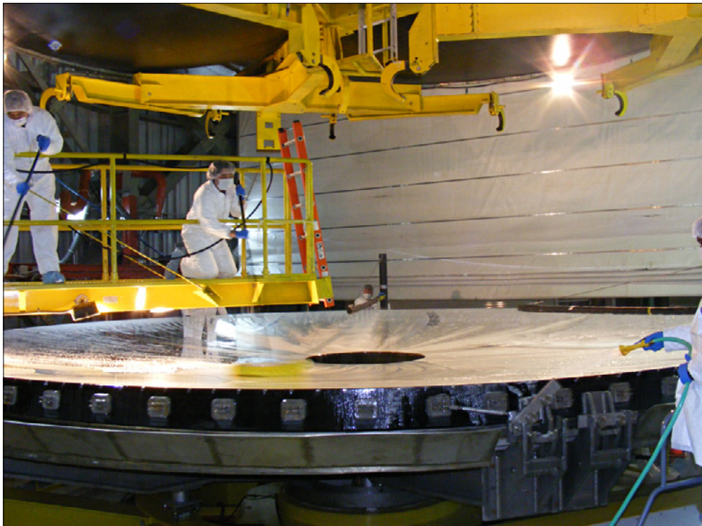
Figure 8. The Gemini primary mirror during cleaning and stripping procedures prior to recoating.
