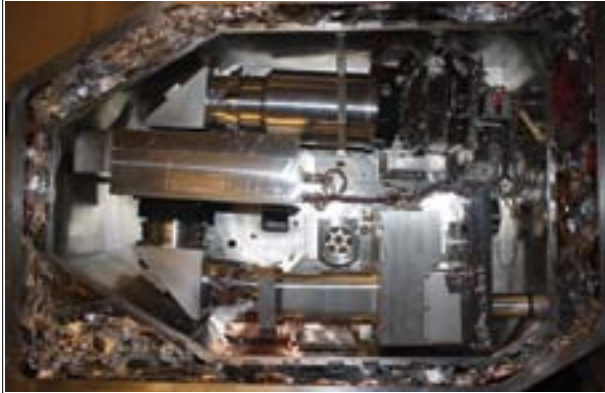
Figure 5. View of the “internals” of the IFS with the dewar lid removed.
