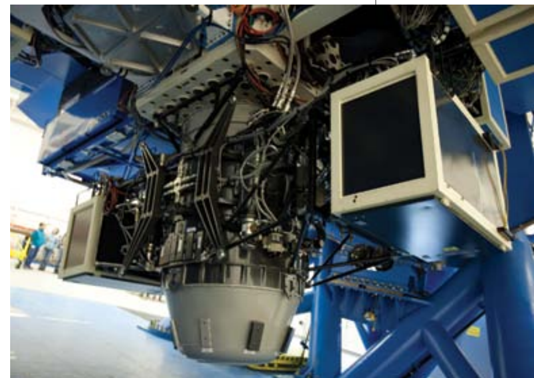
Figure 1. GNIRS mounted on the bottom (uplooking) port of the Gemini North telescope in August 2010.
