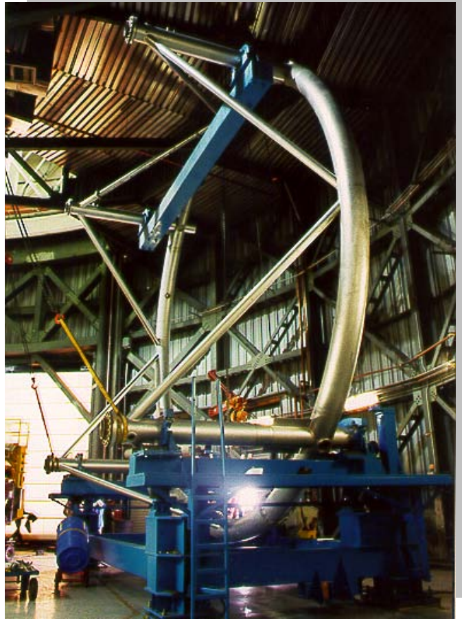
Gemini North Cassegrain rotator in final testing.
