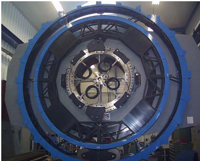
Gemini North Cassegrain rotator in final testing.
