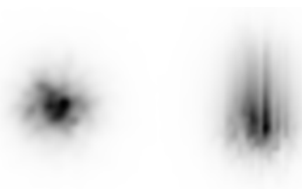
Figure 28: Instantaneous PSF on the tip-tilt sensor at a 45° zenith angle without (left) and with (right) dispersion.
