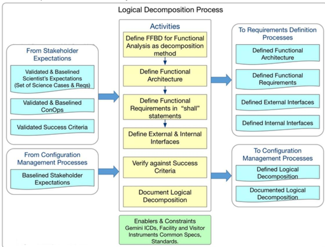
**Figure 4. Logical Decomposition Process**
