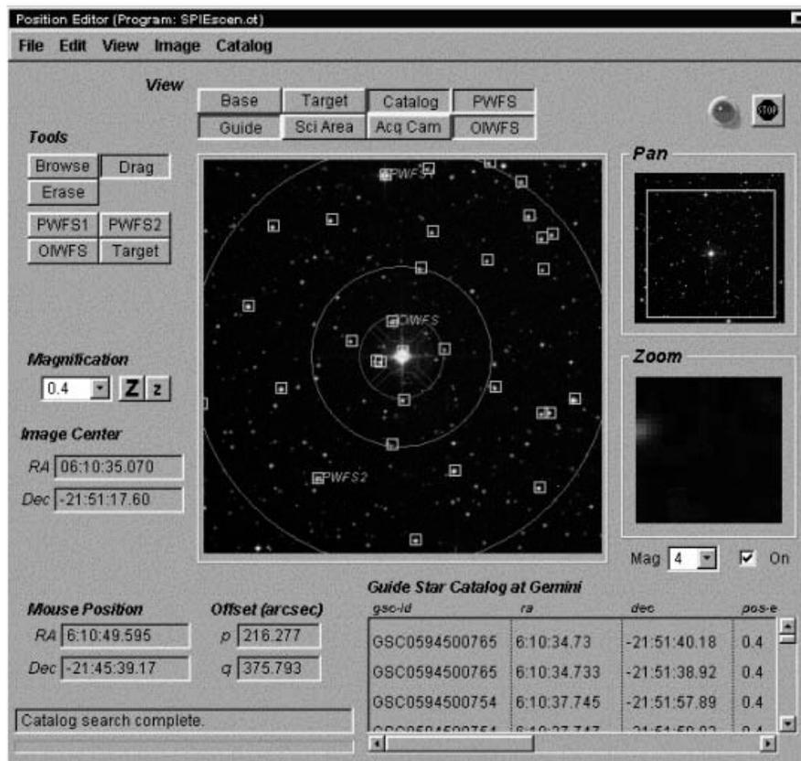
Figure 9: Visual representation showing catalogued guide stars (square boxes), those selected for the wavefront sensors (labelled), and patrol fields for the WFSs: outer circles for the peripherals and inner circle and vignetting pattern for the on-instrument.
