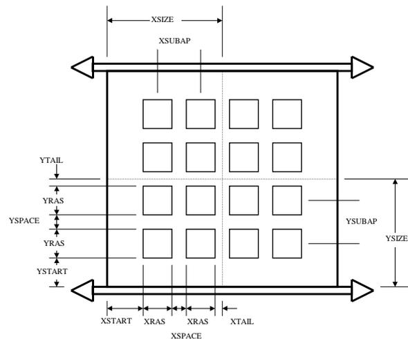
Figure 14. Generalized Readout Geometry
