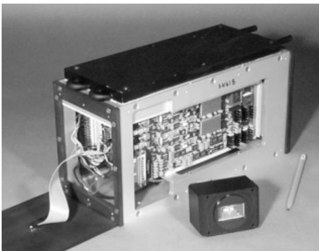
Figure 13. WFS Controller and CCD Housing.
