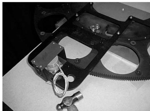
**Figure 17:** Filter Wheel with Motor Mounted
