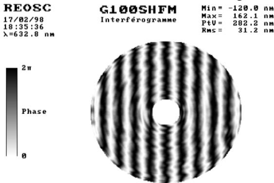
Figure 1. REOSC measuring results for Primary Mirror #1.
