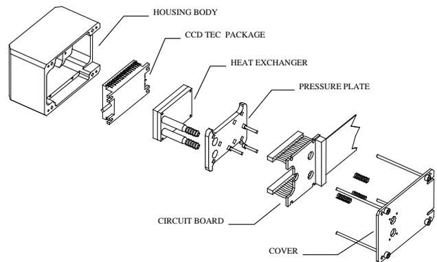
**Figure 12:** WFS CCD Housing
