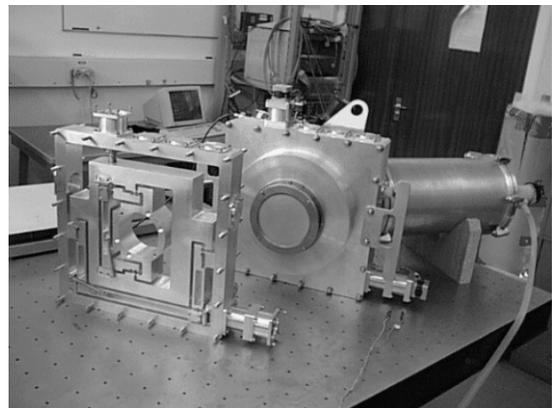
**Figure 16:** x,y,z CCD Translation Stage
