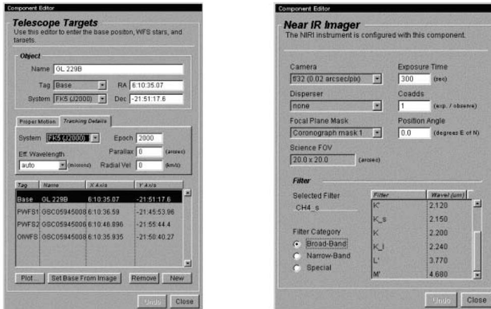
Figure 8: The Observing Tool components used to define (a) the telescope and wavefront sensor positions and (b) the near-infrared imager configuration.
