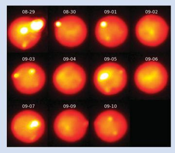
**Left:** NIRI + Altair Natural Guide Star adaptive optics observations of the August 29, 2013, volcanic outburst on Jupiter's moon lo over a two-week period. Due to lo's rotation, a different area of the surface is viewed on each night; the outburst is visible with diminishing brightness on August 29-30 and September 1, 3, and 10. *Credit: K. de Kleer & I. de Pater (2016)*
